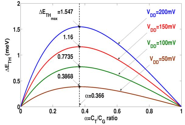
Fig. 7. Variation of quantization threshold  $\Delta E_{TH}$  as a function of  $\alpha = C_T/C_G$  ratio for a noise tolerance of 10% of the orthodox noise margin (i.e.,  $x = 0.1$ ). Note that  $(C_G + C_T)$  value is decreased (considering SET devices with smaller dimensions) proportionally with increase in  $V_{DD}$ .
