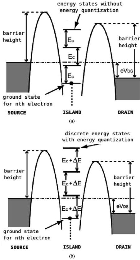
Fig. 1. Schematic of the energy diagram of an SET (a) with and (b) without energy quantization. Here,  $E_c$  is the charging/addition energy. (adapted after [11]).
