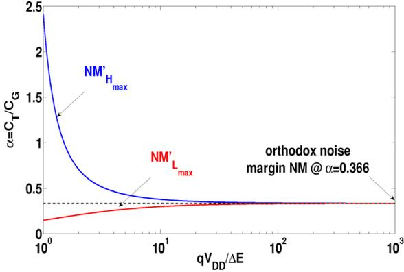
Fig. 8. Variation of  $\alpha = C_T / C_G$  ratio as a function of the ratio  $qV_{DD} / \Delta E$ , indicating the value of  $\alpha$  necessary at a given bias  $V_{DD}$  and energy quantization  $\Delta E$  to obtain maximum noise margins.
