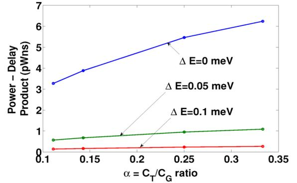
Fig. 5. Variation of power-delay product (in pWns) with capacitance ratio  $\alpha = C_T/C_G$  using different values of energy quantization  $\Delta E$  (in millielectronvolts) as a metric.
