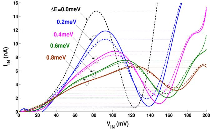
Fig. 9. Influence of energy quantization and temperature on  $I_{IN} - V_{IN}$  characteristics of the NDR circuit. The solid and the broken lines represent the plots at temperatures 40 and 80 K, respectively. The minor dotted lines represent the path followed by the circuit during operation, giving rise to the hysteresis shown in Fig. 10 (simulated for  $I_{BIAS} = 5$  nA,  $R_T = 1$  M $\Omega$ ,  $C_G = 0.5$  aF, and  $C_T = 0.25$  aF).
