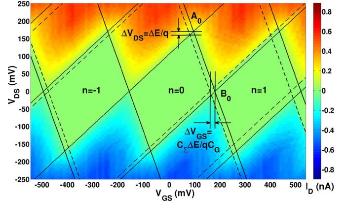
Fig. 2. Influence of energy quantization on  $V_{DS} - V_{GS}$  surface characteristics (drain current contour) of an SET. The solid and broken lines represent the solution of  $\Delta F = 0$  for quantized ( $\Delta E = 10 \text{ meV}$ ) and continuous ( $\Delta E = 0$ ) energy levels in the island, respectively. (simulated for  $R_T = 1 \text{ M}\Omega$ ,  $C_G = 0.5 \text{ aF}$ ,  $C_T = 0.25 \text{ aF}$ , and temperature  $T < q^2/k_B C_\Sigma = 90 \text{ K}$ ).
